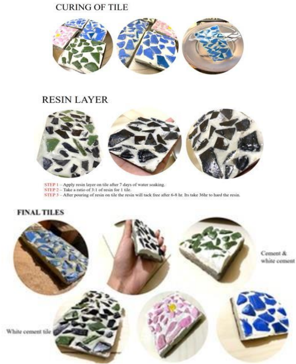
Figure 3: Shows the Final Structure of Tile
